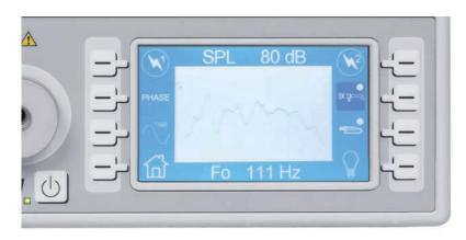
The angle of the LED flash in Phase mode (0-400°) can be modified through the powerful software and the pedal, as well as the flash speed in Slow motion (0.5-2Hz), providing hands-free operation.
