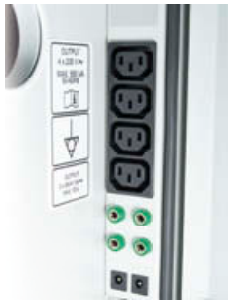
8-SOCKET INTERNAL SAFETY CONNECTION (4 ON EACH SIDE)
